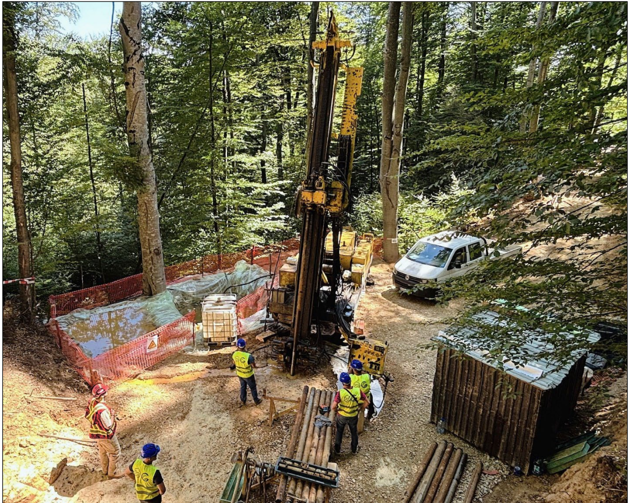
Figure 5. Drill pad BRE23005 with the rig oriented at 345 azimuth and inclined at 70° to surface testing the deep conductor interpreted to be the previously intercepted Sb-Ag-Zn mineralization.
